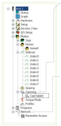
**Camming** – Cams make set-up and programming of complex motion profiles easy. The use of real-time programs provides smooth transitions when switching between cam profiles on-the-fly. Cam data is easily imported within PowerTools Pro and the cam graphing tool features multiple interpolation types.
