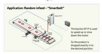
Refer to Figure 2. Up to 8 outputs can be triggered to "ON" based on motor or master encoder position range that is affected by motion in one direction, both directions or rotary rollover. Another mode of the PLS allows the output(s) to be triggered by time.
